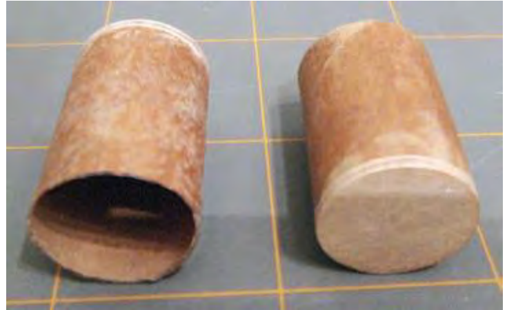
Two piston heads made from coupler stock and bulkhead disks.
