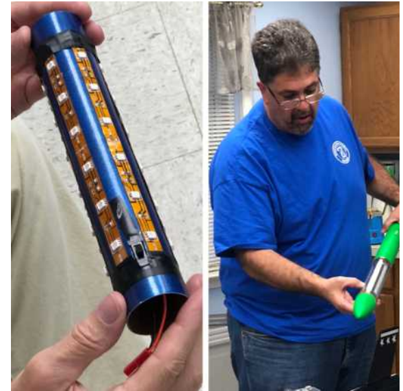
Right: Jim Filler showed his night rockets. They use a cylinder bedecked with LED strips. The cylinder then fits inside a model's clear payload section and connects to a LiPo battery.
